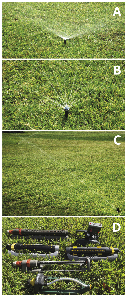
Figure 4. Different types of sprinklers: A) spray head, B) multi-stream rotary, C) rotary, and D) hose-end.
